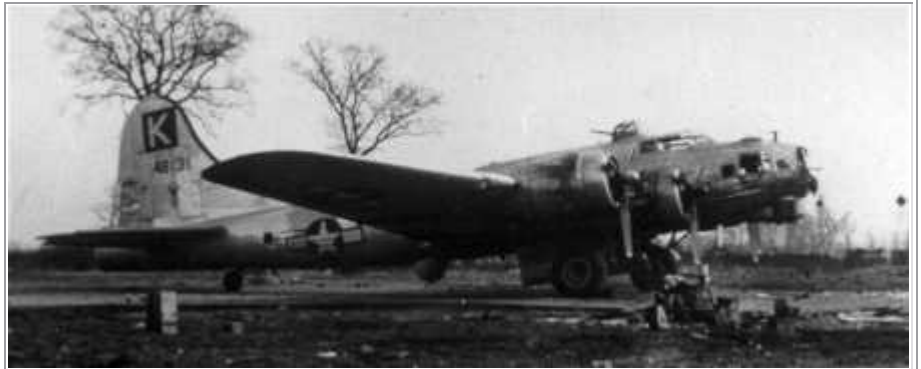
44-8131 Y (name unknown) PFF Photo dated Feb. 22, 1945 H2X pathfinder. Damaged in the explosion and fire at Rattlesden on February 21, 1945; written off and salvaged.
